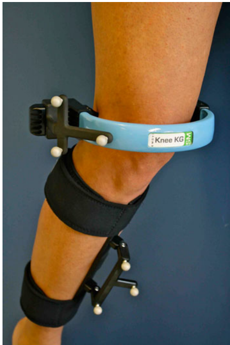
Fig. 1 Anterior view of a right knee fitted with the KneeKG tracker system. Secure fixation to the thigh and calf minimizes skin motion artifact
