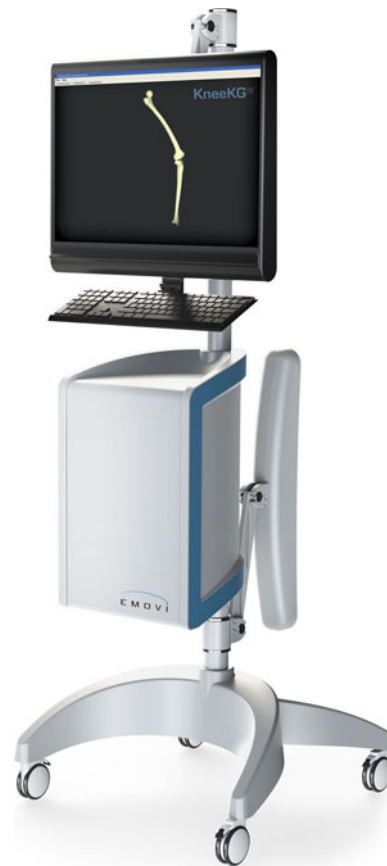
Fig. 2 The KneeKG TM is composed of an infrared motion capture system (Polaris Spectra camera, Northern Digital Inc.) and a computer equipped with the Knee3D software suite (Emovi, Inc.). The camera and computer can both be mounted on a cart making the entire system mobile
